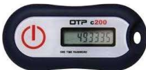
Picture 7: The example of a hardware token generating one time passwords
